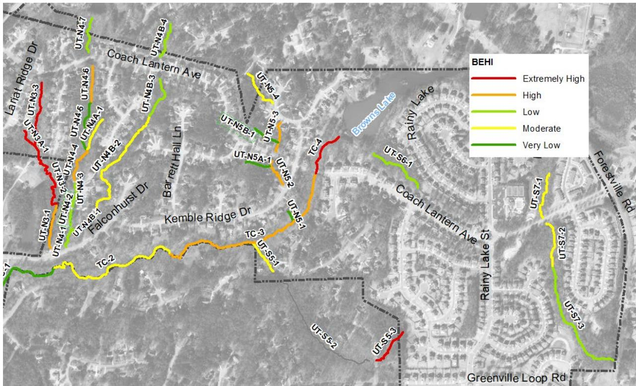
Figure 10. Erosion Hazard Rating Map
